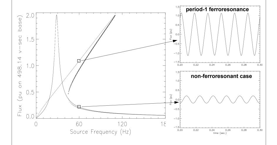
fixed parameters: C=12450 pF, R=2.5 M $\Omega$ , E=0.167 pu, L=2500 H,  $a_1$ =0.1,  $a_3$ =1.0
