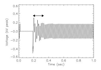
FSC Enabled: transients damp within 10 cycles
