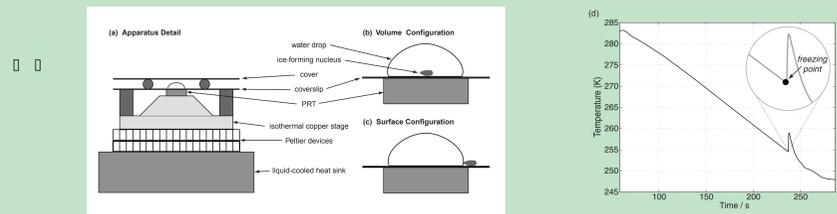
Figure 1. (a) Apparatus detail; (b) Volume configuration; (c) surface configuration; (d) example temperature curve from a cooling cycle.
