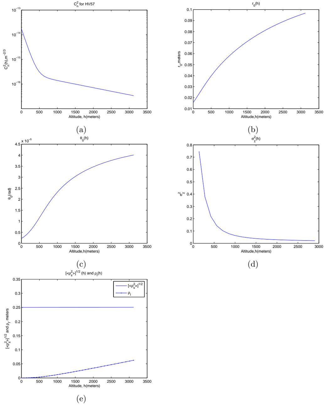
**Figure 1.** Structure constant  $C_n^2$  and beam parameters as a function of altitude,  $h$ : (a) Structure constant  $C_n^2$ ; (b) Fried parameter  $r_0$ ; (c) Isoplanatic angle  $\theta_0$ ; (d) Rytov variance  $\sigma_\chi^2$ ; (e) Isoplanatic patch radius  $\rho_I$  and Mean square instantaneous spot radius in the target plane  $\langle \rho_s^2 \rangle$
