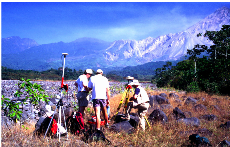
Fig. 3. The kinematic GPS base station for surveying debris flow volumes. Santiaguito volcano is in the background. From left to right: Luke Flynn, Mark Davies, and Gregg Bluth.
