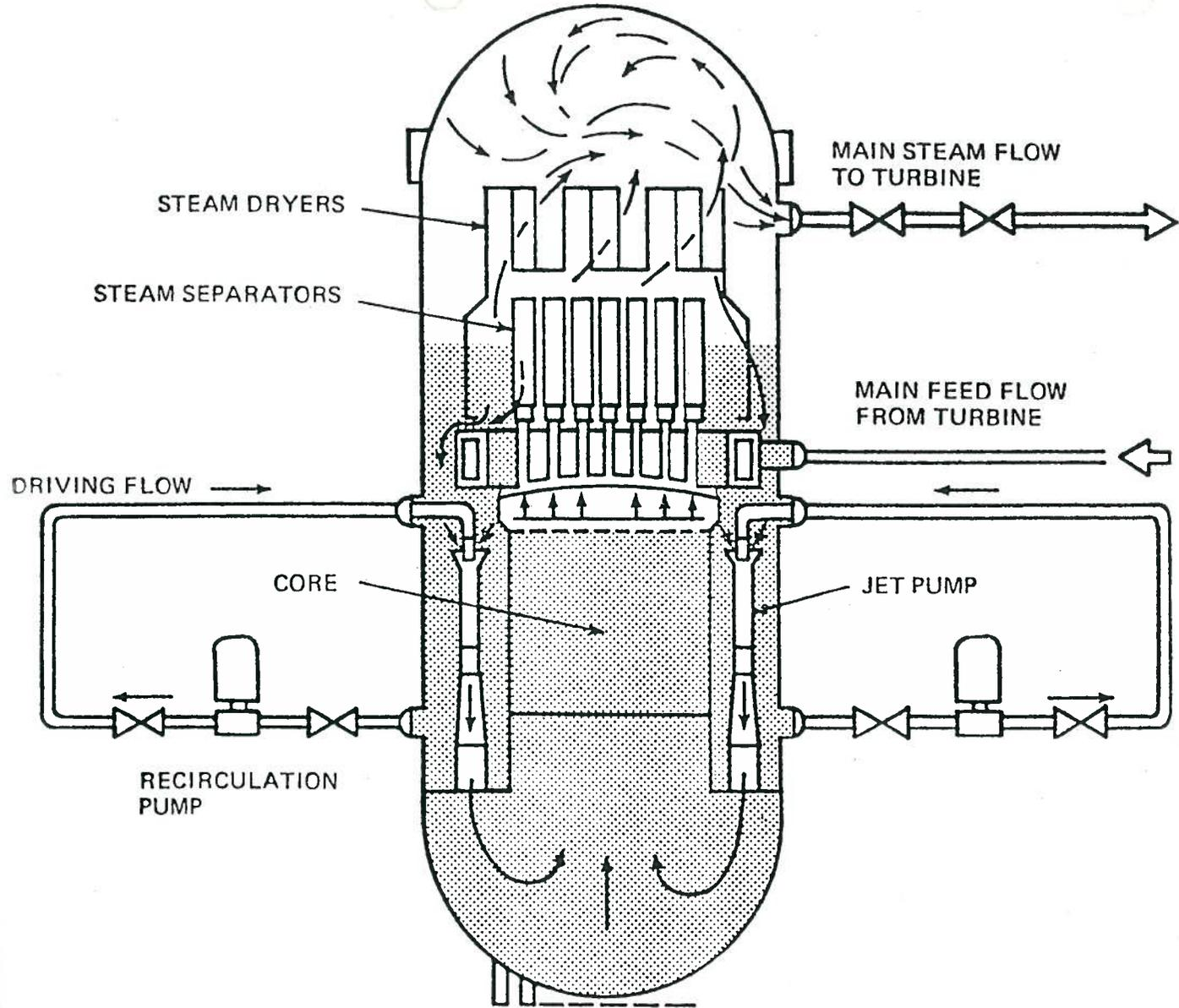
Figure 10-17 BWR reactor vessel internal flow paths.
