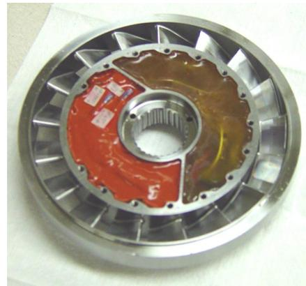
**Figure 5. Stator with cover removed to show telemetry electronics installed in the hub.**
