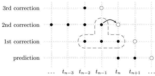
FIG. 2.2. This plot shows the staggering required for a fourth order RIDC scheme (RIDC4-BE), constructed using backward Euler predictors and correctors. The time axis runs horizontally, and the correction levels run vertically. The white circles denote solution values that are computed simultaneously, e.g., core 0 is computing the prediction solution at time  $t_{n+2}$  while core 1 is simultaneously computing the 1st correction solution at time  $t_{n+1}$ , etc.
