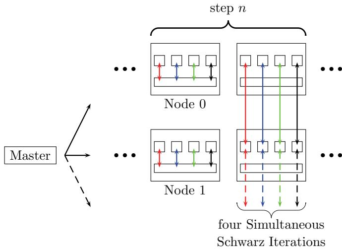
FIG. 3.1. RIDC framework for time integration with a classical Schwarz iteration in space. For this RIDC4-DD illustration, it is assumed that each node, working on a subdomain, has four cores with access to shared memory. After an initial start-up period, each step consists of updating the memory footprint, followed by four simultaneous Schwarz iterations.
