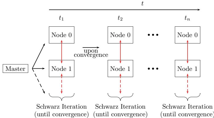
FIG. 2.1. Communication diagram where backward Euler is used to integrate in time with a classical Schwarz iteration in space.
