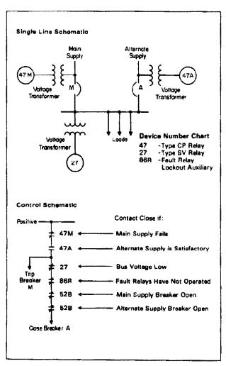
Figure 6-26: Bus Transfer Schame Utilizing Polyphase Voltage Relays.
