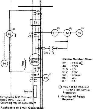
Figure 6-25: Recommended Potection for Small Generators as Used in Industrial Plants.
