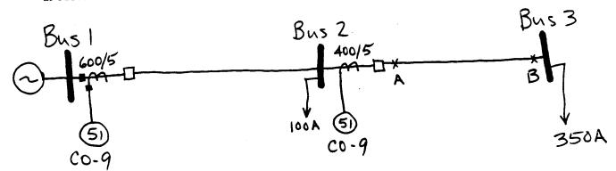
a) Determine the tap settings for the relays at buses 1 and 2. Assume that taps can be set so they are just above rated load current. Available tap settings are: 1.0, 1.2, 1.5, 2.0, 2.5, 3.0, 3.5, 4.0, 5.0, 6.0, 7.0, 8.0, 10.0, and 12.0 amps.
