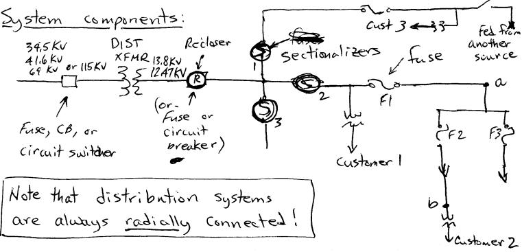
Recloser - combined relay/CT/circuit breaker. Usually attempts 2-4 recloses following a fault. Sectionalizer - switch that automatically disconnects after set number of fault/trip events. Set to disconnect after one less than max reclose attempts. Ex: 4 reclose attempts -> lockout sectionalizer after 3 fault surges.
