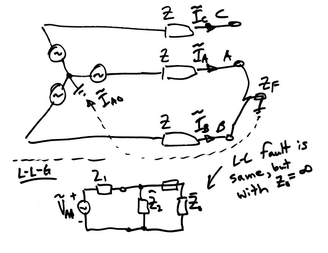
IF ZTH+ZLIKE TLOND ⇒ ZLOAD determines S.S Φ-angle of I. => ZTH+ZLINE determines of I during fault!
