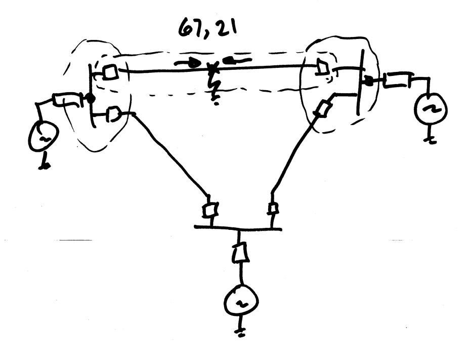
Grid & Holo Cew John Grid Area V2 (A) V2 (A) Z  $\frac{P_{12}}{\sqrt{2}} = \frac{V_1 V_2}{\sqrt{2}} \sin (\alpha - \beta)$ (d-b) increases as P12 increases -Tripping line increases LSI-LB - Reclosing may be problematic...?? 67-Directional O.C. (Can also have inst. & time delay versions).
