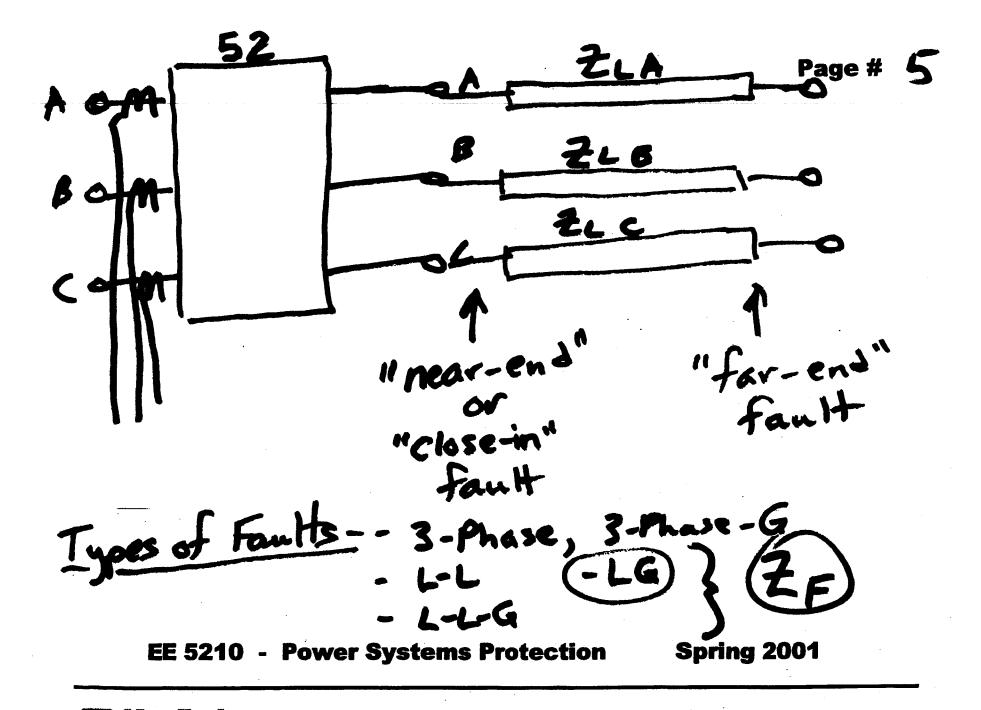
Ref: Tables 4,34 \$ 4,35 ! GND Relay located at sending (near) and - Voltage at relay greatly reduced during fautt, but will only be zero for close-in fault.
