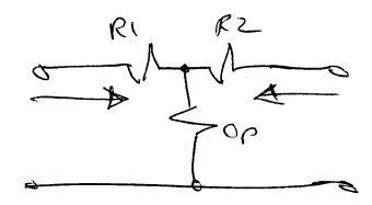
IA87 is wired reverse polarity (it should be 180 degrees out of phase with IA). IB87 is really reverse polarity IC87 (it should be 180 degrees out of phase with IB and 120 degrees behind IA87).
