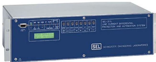
Figure 5: SEL311L line current differential protection
