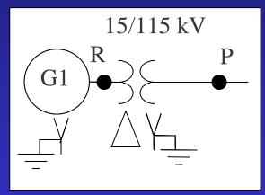
G: 100 MVA, 15 kV Transformer:
