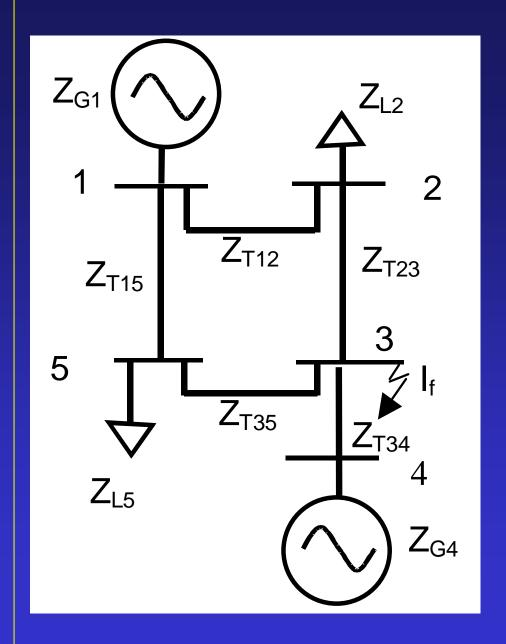
How do you calculate the fault current  $(I_f)$  at bus 3?
