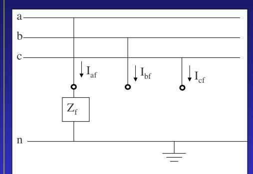
Fig.1. Single line to ground fault on phase A
