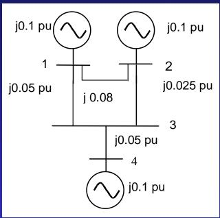
$$Z_{\text{bus}} = j \begin{bmatrix} 4.783 & 3.044 & 3.261 & 2.174 \\ 3.044 & 4.534 & 3.634 & 2.422 \\ 3.261 & 3.634 & 4.658 & 3.106 \\ 2.174 & 2.422 & 3.106 & 5.404 \end{bmatrix} \times 10^{-2} \text{ pu}$$
