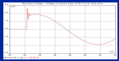
Peak Bus Voltage = 1.4 per unit, Frequency = 5 KHz.
