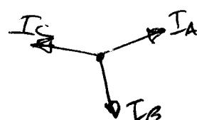
b)  $V_{LL} = 69 \text{ kV RMS}$ . The load consumes 300 MVA at a PF of 0.8 LAG. Calculate the phasor value of  $I_A$  flowing into the load.
