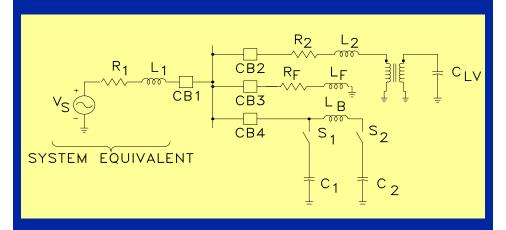
CB1 Closed, Fault on Bus. Open CB1 to Clear Fault.
