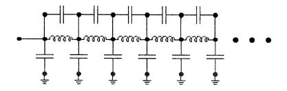
With high frequency waves, series capacitance forces uneven voltage distribution. Terminal end sees highest voltage.
