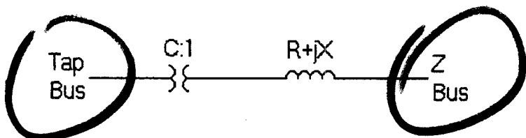
**Complex turns ratio due to phase shifting
