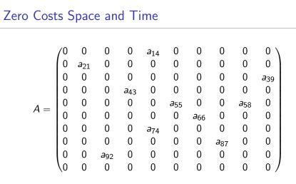
Storing every double-precision element requires 800 bytes Storing only non-zero double-precision elements requires 80 bytes
