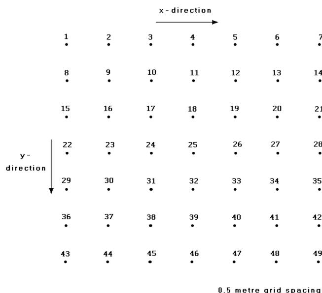
Figure 34. Arrangement of electrodes in the Birmingham 3-D field survey.
