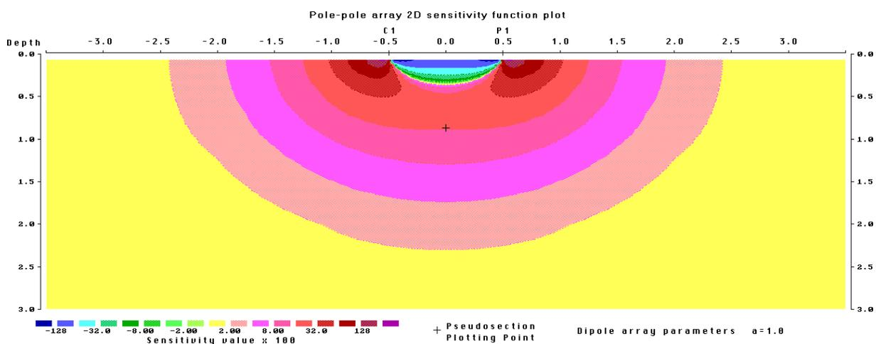
Figure 11. The sensitivity pattern for the pole-pole array.
