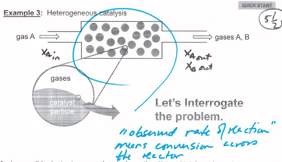
An irreversible, instantaneous chemical reaction  $(2A \rightarrow B)$  takes place at a catalyst surface in a reactor as shown. How might mass transfer affect the observed rate of reaction?
