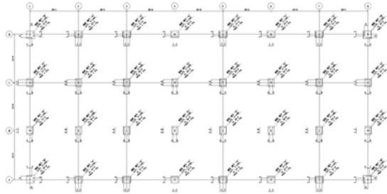
One of the first drawings prepared by the detailer is the anchor rod plan. This plan guides the foundation subcontractor in the placement of anchor rods. It contains horizontal and vertical information for placement of anchor rods, as well as dimensions and elevations of leveling plates (if used).
