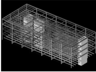
The following is an animation of the structural steel erection process by sequence. The six sequences will slowly appear along with the working day in which hoisting of each sequence was completed. The last images to appear are of the masonry stair and elevator shafts. They were built after the frame was erected. The steel frame was connected to the vertical shafts to provide permanent lateral stability of the frame.
