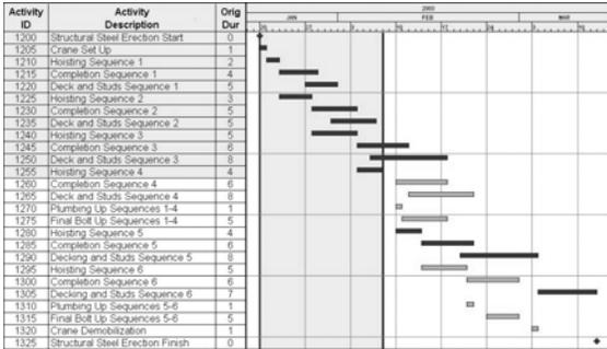
The activities in yellow are the ones completed by the time sequence 4 was hoisted. Notice that deck and studs for sequence 3 were started before hoisting sequence 5 in order to provide fall protection for the ironworkers connecting steel. Plumbing up and final bolt up for sequences 1 through 4 were performed after sequence 4 was hoisted.
