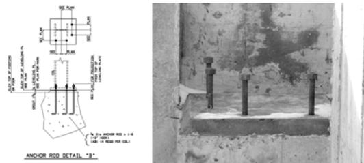
The anchor rod detail on the left depicts how anchor rods and leveling plates were placed for the case study project. A leveling plate is a steel plate fixed on top of a foundation on which a structural column can be placed. The leveling plate is leveled and grouted prior to installation of the column. Although this is one method for setting columns, practices may vary with other erectors. On the right is a photograph of the anchor rods and leveling plates in place for the case study project.
