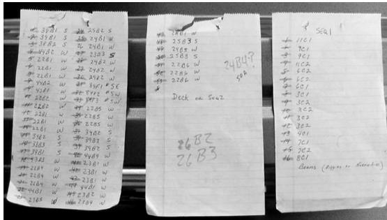
The erection crew foreman used the erection drawings to determine the exact order in which structural steel members were to be erected. The first pieces hoisted during this project were the columns in sequence 1 (right sheet), then girders and beams (left and center sheets).
