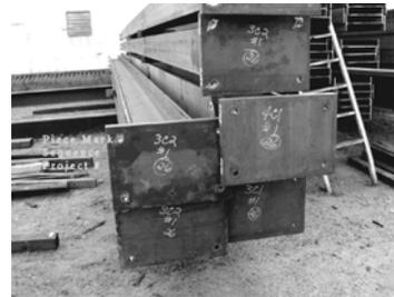
Once fabricated, each finished structural steel member is labeled. In this case the fabricator labeled each steel member with its piece mark, sequence number, and the last two digits of the job number. Specific labeling practices may vary by fabricator. Notice that this time the label color is yellow to differentiate it from previous labels. Labeling of the steel pieces is crucial because it will help identify members on the job site.
