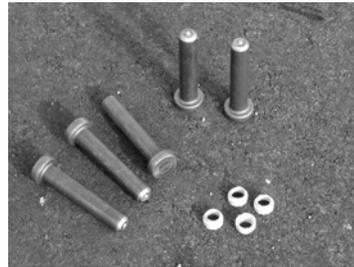
These are shear studs. The white rings are ceramic ferrules. The ceramic ferrule constrains the molten metal into which the stud is thrust automatically and a high quality fusion weld is accomplished where the weld is stronger than the stud itself.
