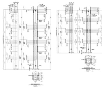
These are shop drawings of columns 3C1 and 3C2 for the case study project. Shop drawings convey precise information to the fabricator, and other project parties about how each steel member in the structure is to be fabricated.
