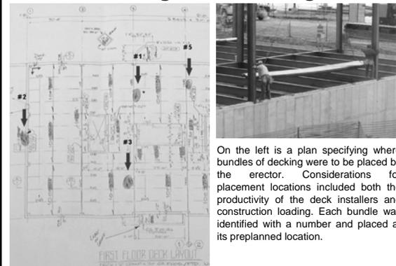
On the left is a plan specifying where bundles of decking were to be placed by the erector. Considerations for placement locations included both the productivity of the deck installers and construction loading. Each bundle was identified with a number and placed at its preplanned location.
