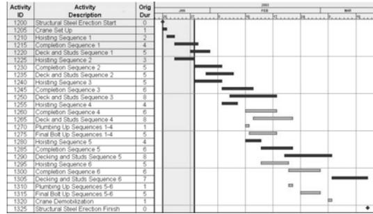
The activities in yellow were completed by the time sequence 2 was hoisted. Notice how deck and studs for sequence 1 starts before hoisting sequence 3 to provide fall protection for the ironworkers connecting steel.
