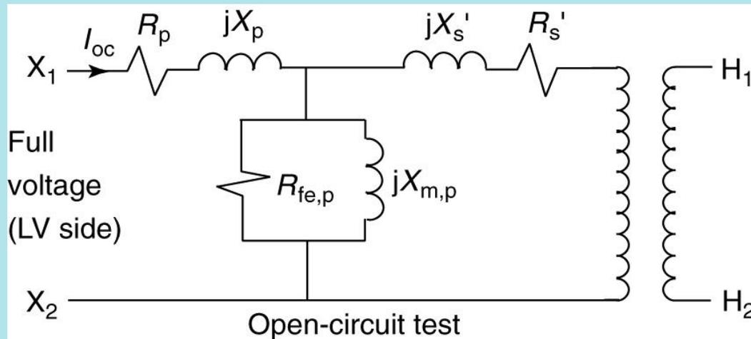
The input impedance during open-circuit test is the primary winding in series with the exciting branch:
