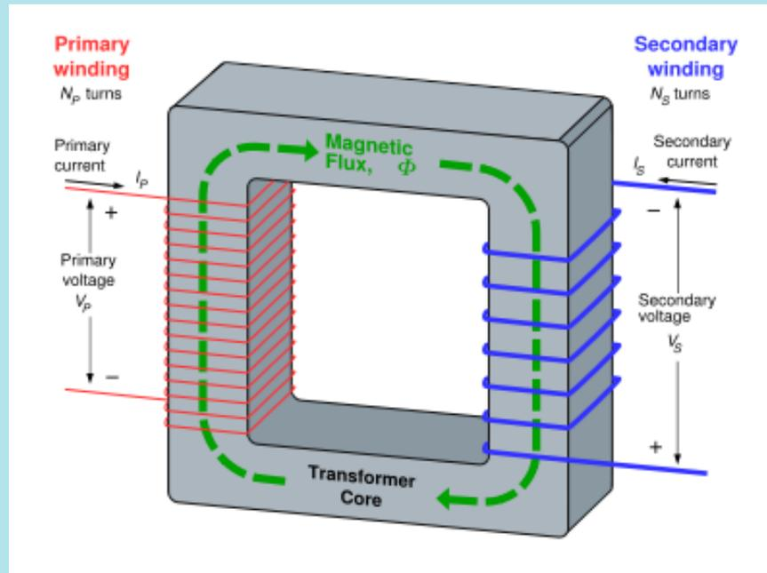
A simple transformer consists of two electrical conductors called the **primary winding** and the **secondary winding**. If a time-varying voltage  $V_P$  is applied to the primary winding of  $N_P$  turns, a current will flow in it producing a [magnetomotive force](#) (MMF).
