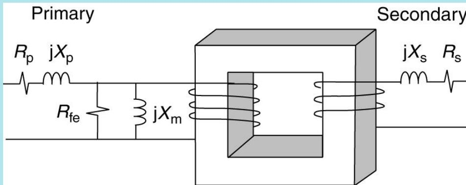
The transformer is now **ideal** and the circuit elements account for the losses and voltage drops in the real transformer.
