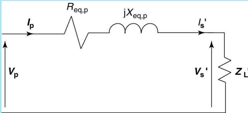
The transformer windings have impedance so there will be a voltage drop across them that changes with current.
