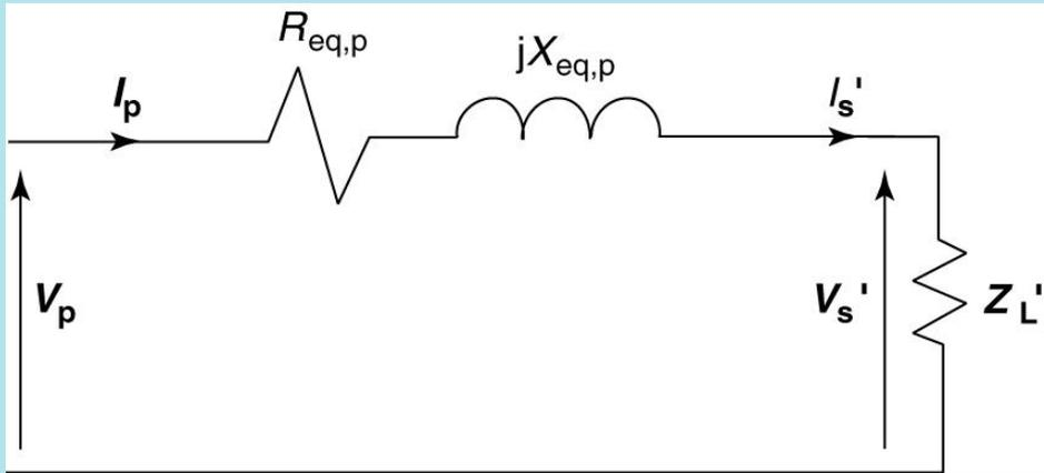
If we know the primary voltage and the current, we can calculate the secondary voltage:
