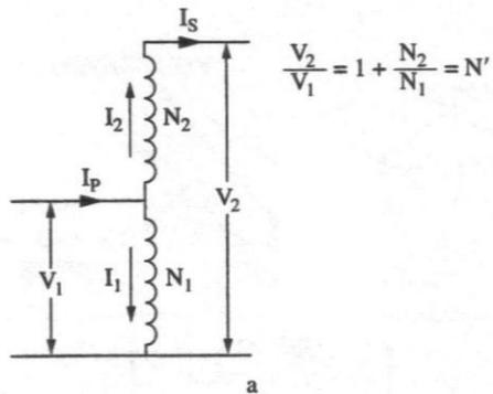
$$\frac{S_A}{S_I} = \frac{I_1 V_1}{I_p V_1} = \frac{N' - 1}{N'}$$
