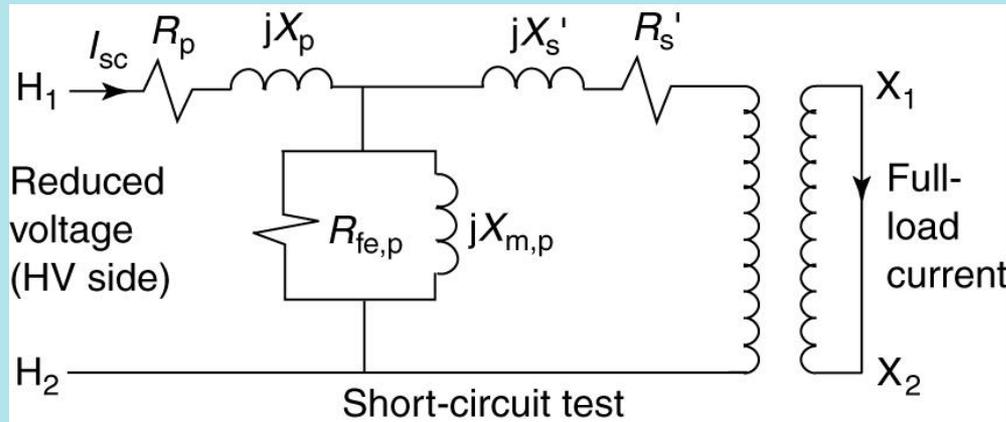
**Technique:** the low-voltage side of the transformer is shorted and voltage is applied to the high-voltage side, because it only takes about 4%-7% of rated voltage to cause rated current to flow in the winding. The measurements are used to calculate value of  $R_{eq}$  and  $jX_{eq}$ .
