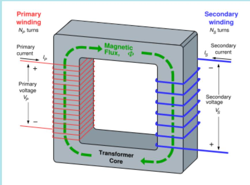
With perfect flux coupling, the flux in the secondary winding will be equal to that in the primary winding, and so we can equate  $\Phi_P$  and  $\Phi_S$ .
