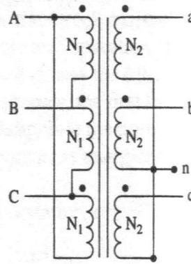
There is a 30 degrees phase shift in both connections. United States industry convention is to connect the secondary so it lags the high voltage primary by 30 degrees.
