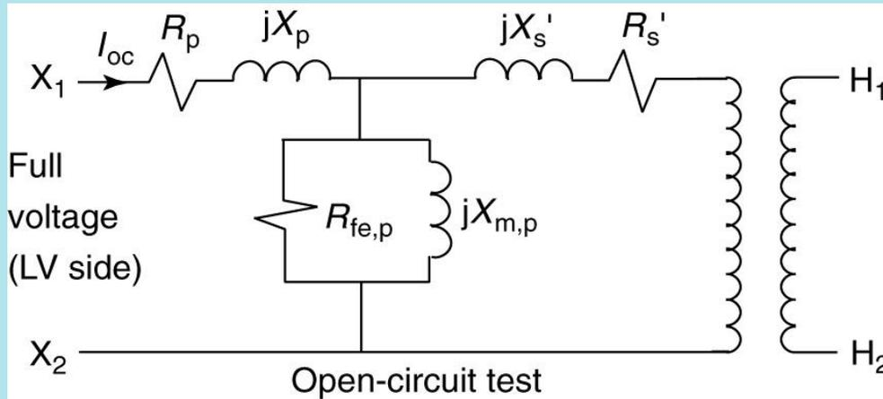
High-voltage side is opened and rated voltage is applied to the low-voltage side (primary side).
