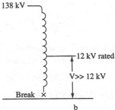
Autotransformers are one winding transformers that are often used in transmission and sub transmission substations.
