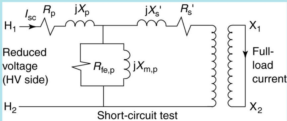
To conduct the short-circuit test:
