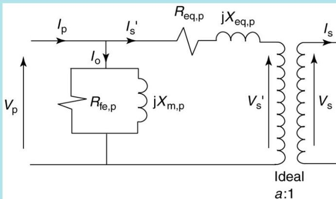
$$R_{eq.primary} = R_p + a^2 R_s = R_p + R'_s$$
