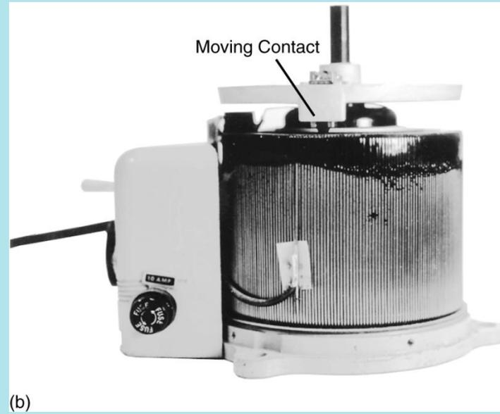
Photograph of an autotransformer for variable-voltage control in the lab.
