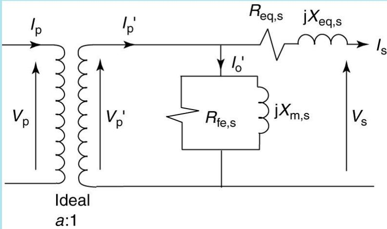
Cantilever circuit referred to the secondary.
