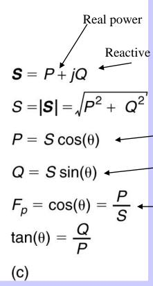
Reactive power Magnitude of the complex (apparent) power Relationship between the real and apparent power. power.
