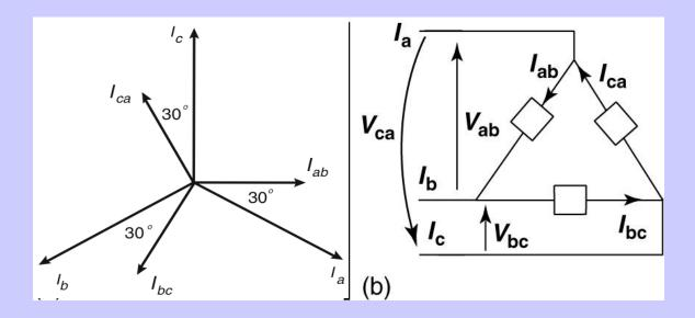
The angular relationship between the line and phase current in a delta system and the relationship of their magnitudes:
