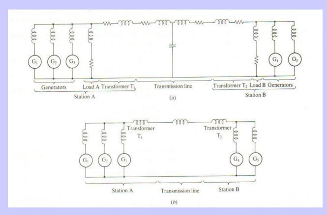
The one-line diagram serves as the basis for a circuit representation that includes the equivalent circuits of the components of the power system.
