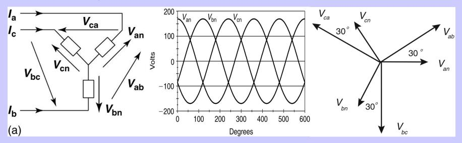
Positive ABC phase sequence (phasors are assumed to rotate in the counterclockwise direction)
