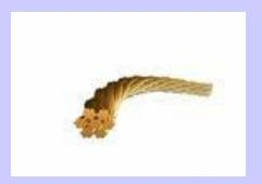
It consists of a number of insulated wire strands woven together in a carefully designed pattern, so that the overall magnetic field acts equally on all the wires and causes the total current to be distributed equally among them.
