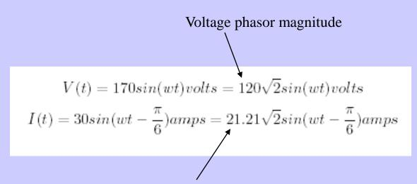
Current phasor magnitude; current is lagging the voltage by 30 degrees
