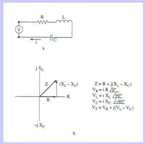
Z – total impedance X<sub>L</sub>- inductive reactance X<sub>C</sub>- capacitance reactance The relation between apparent, reactive, and real power:
