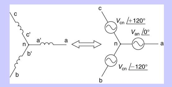
Example: 3-phase generator contains coils that are physically spaced 120 degrees apart and when the rotor turns, the voltages induced in the coils are electrically 120 degrees apart.
