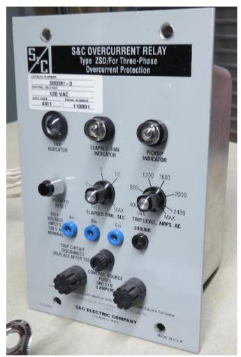
Figure 3: Photograph of subject relay from Bay 8 during bench testing after the outage.
