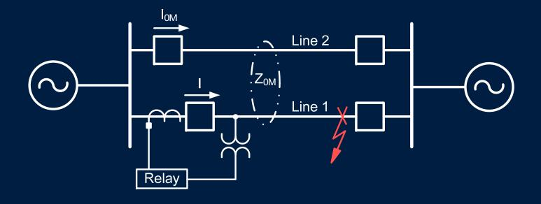
$$Z_{APP} = \frac{V_{a}}{I_{a} + k_{0}I_{r}} = mZ_{1L} + mZ_{0M} \frac{I_{0M}}{(I_{a} + k_{0}I_{r})}$$
