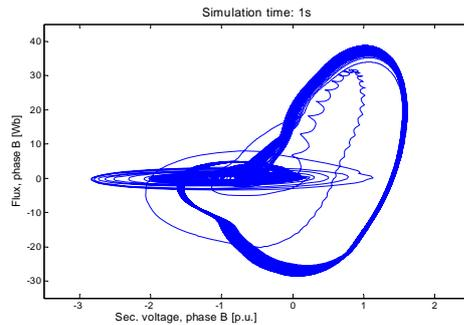
Figure 6 : Flux over secondary voltage, phase B; simulation time of 1 s
