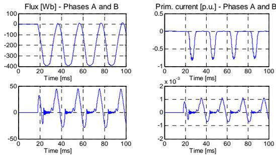
Fig. 5: Fluxes and primary inrush currents - Phases A and B
