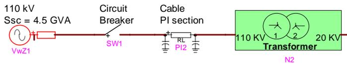
Fig. 1: Simplified drawing of the considered network configuration.
