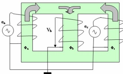
Fig. 2.a: transformer magnetic core
