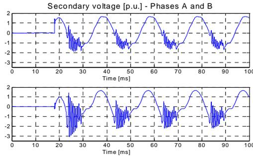
Fig. 4: Overvoltages at the secondary windings of the target transformer- Phases A and B.
