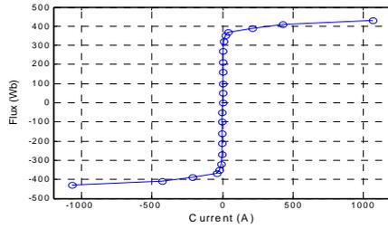
Fig. 3: Non linear characteristics of the target transformer.
