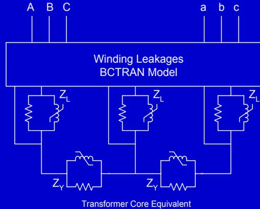
**BCTRAN model for a three-phase three-legged stacked core transformer**
