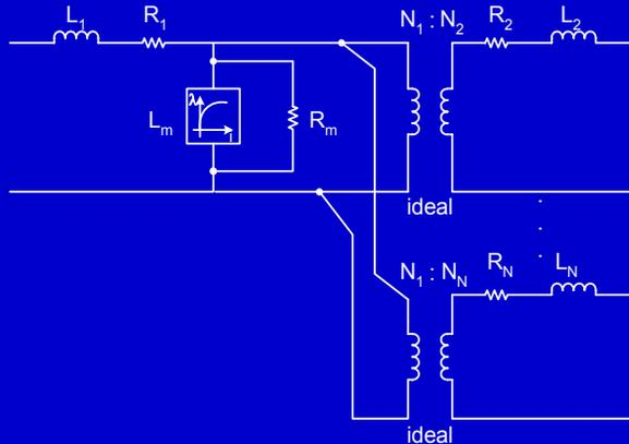
Star-circuit representation of single-phase N-winding transformers
