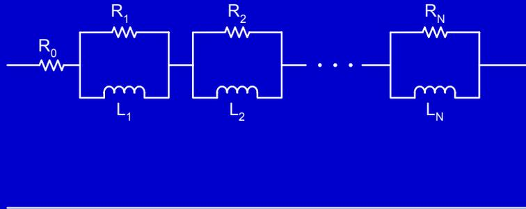
Series Foster equivalent circuit
