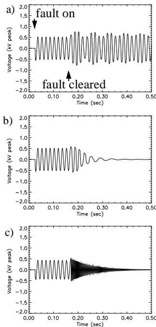
Fig. 9. Example of voltages oscillations across open-delta with 15000 pF, a) no mitigation, b) 83 ohm resistor (25% of PT thermal rating), c) GB connected.
