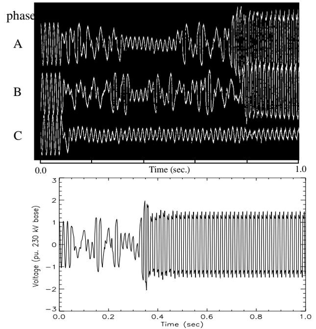
Fig. 2. Benchmark case results. Top: recording. Bottom: EMTP.
