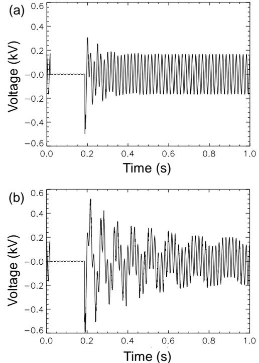
Fig. 11. CSA ferroresonance test comparison with, (a) ferroresonance suppression circuit (FSC) enabled and with, (b) FSC disabled.
