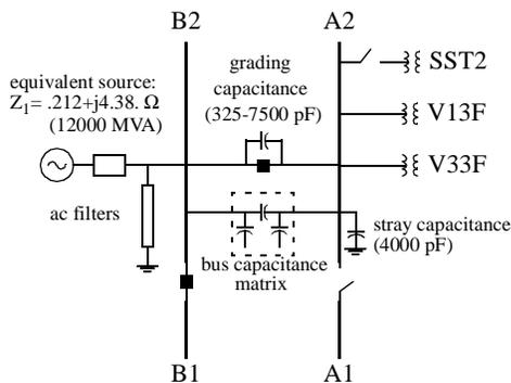
Fig. 1. Wound PT circuit model single line diagram.
