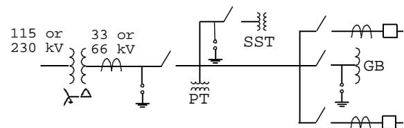
Fig. 8. Typical station layout.
