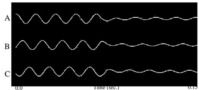
Fig. 3. Trip testing with 200 ohm resistors. Bus A2 voltage.
