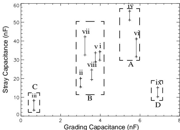
Fig. 7. Dorsey station service transformer stray and grading capacitance operating environment.
