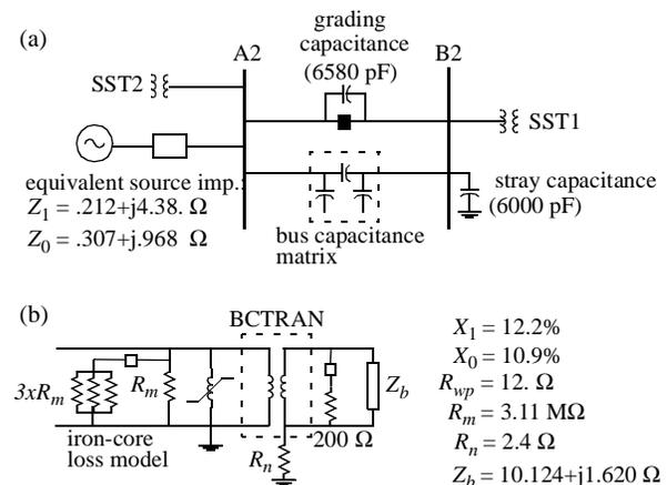
Fig. 5. Single-line diagram of the August 5, 1995, Dorsey disturbance showing (a) main circuit components and (b) model of station service transformer.
