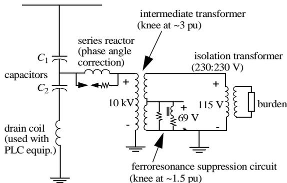
Fig. 10. Typical CVT single line diagram.
