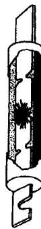
(b) The link melts and an arc is established under sustained overload current
