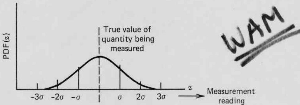
FIG. 12.8 Normal distribution of meter errors.
