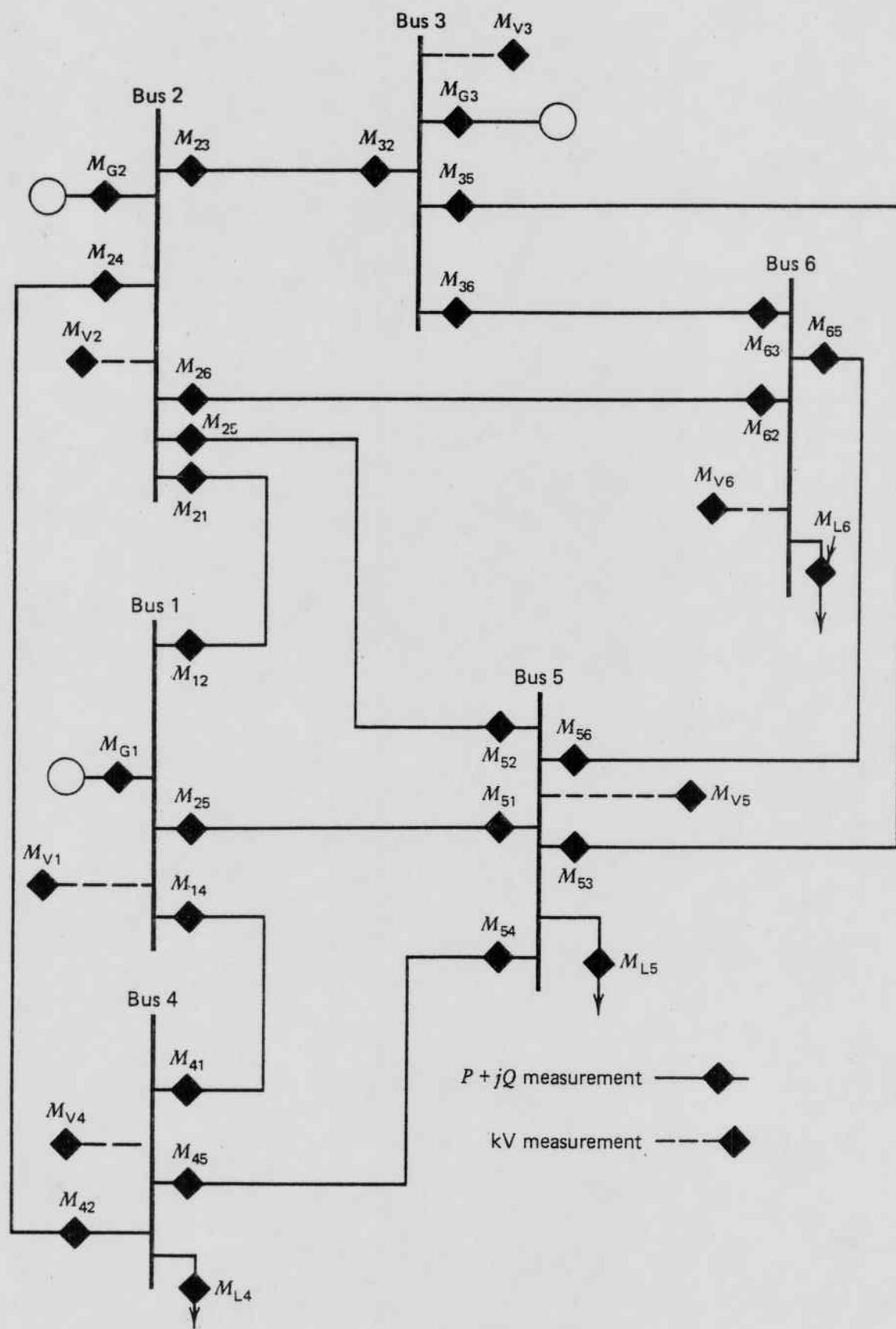
FIG. 12.12 Six-bus system with measurements.
