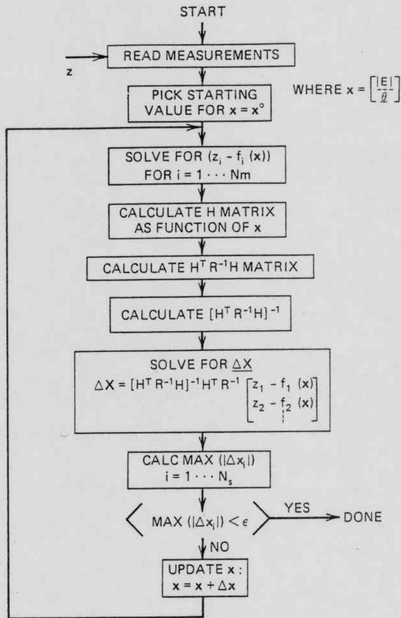
FIG. 12.11 State estimation solution algorithm.
