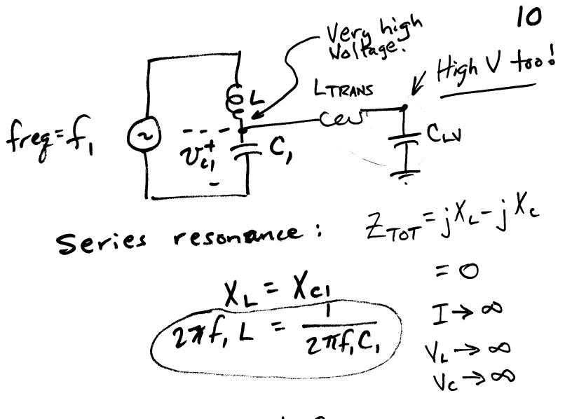
Per Unit Voltage at CLV is higher than at CI, thus the name "Voltage magnification."
