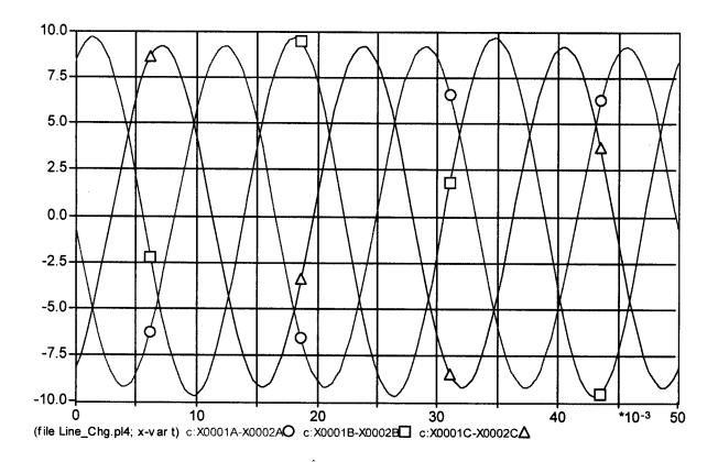
As predicted, phase B line current is larger than A or C, due to larger capacitive coupling to phase B. Larger capacitive effect ==> smaller input impedance ==> higher current...
