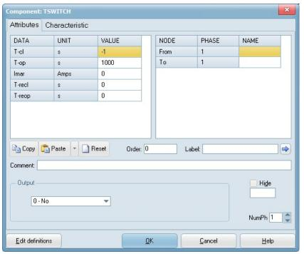
Here you can see the default timecontrolled switch. One close time and one open time.
