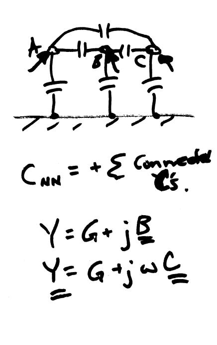
Line Charging Example: LCC\_3b.alc (Coupled-PI, 60 Hz model).
