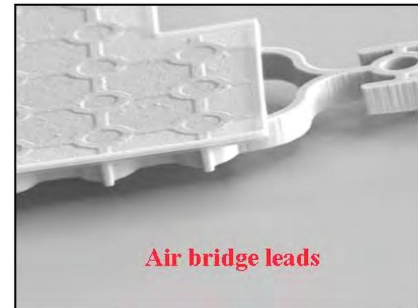
Linear ion trap chip micro-fabricated with a metal MEMS process at Sandia National Laboratories. Planar metallic trap electrodes (W overcoated with Au) and a hole through the Si substrate define the trapping region and allow 3D optical access for lasers to ions trapped between RF leads stretched lengthwise over the hole. Control electrodes at the hole edges define seven trapping segments. Air bridge metal leads reduce capacitance and RF dissipation to the substrate.
