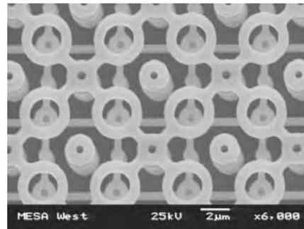
The process is low temperature (CMOS compatible), and can be used to fabricate highly complex structures from dielectrics and tungsten
