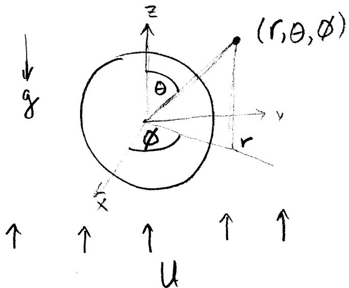
We "fix" the  $r, \theta, \phi$  coordinate system to the falling sphere.  $u$  appears to the sphere as a uniform constant velocity field at steady state (when drag force = gravity force).
