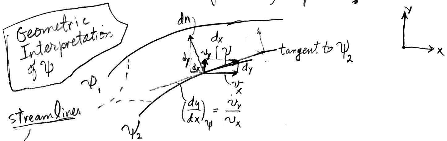
Thus, the flow path within the fluid are along paths of constant  $\psi$ , thus the Stream Function is valuable for flow visualization.
