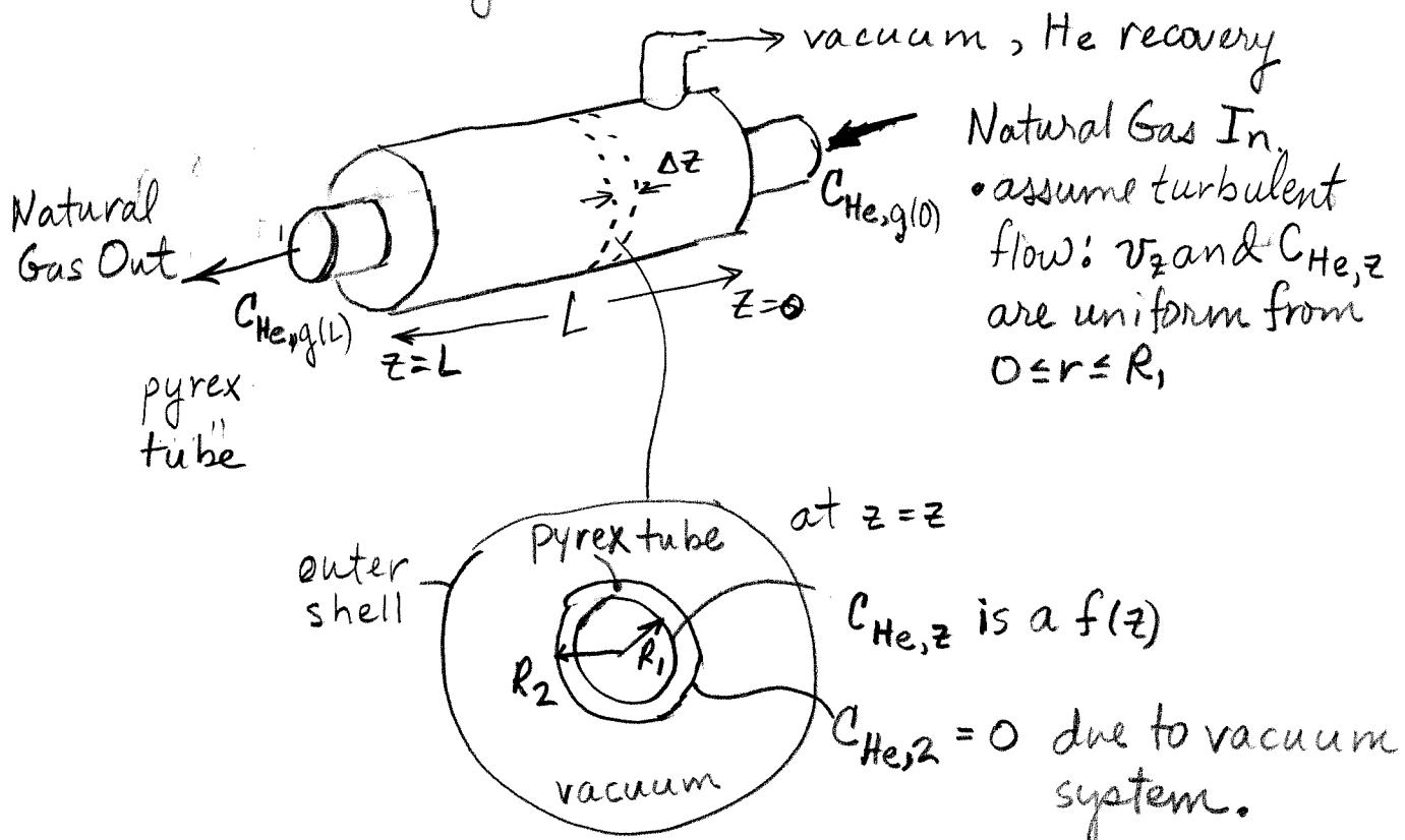
Shell Balance in Pyrex Tube: steady-state
