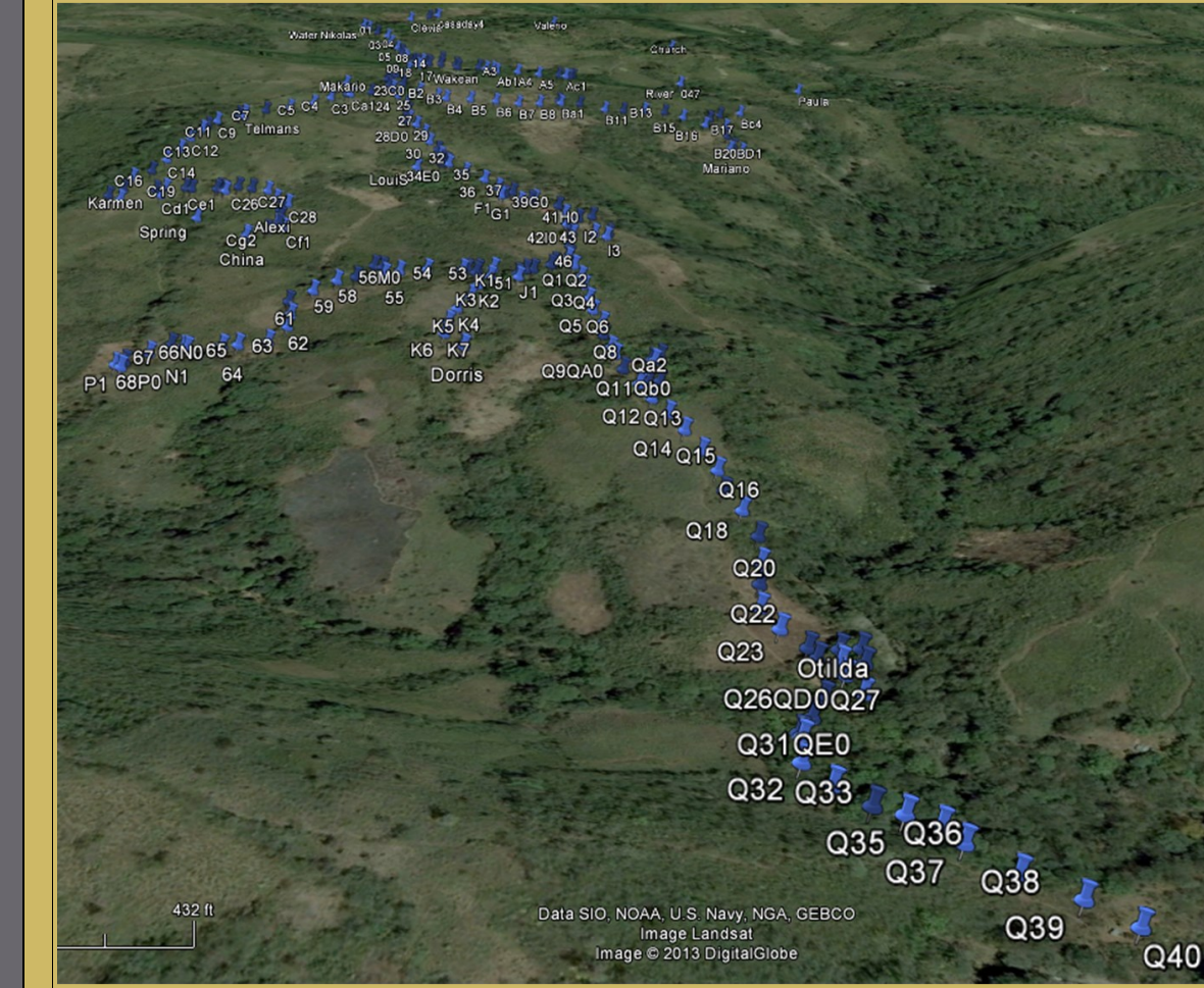
Figure 3: Survey route of proposed pipeline.
