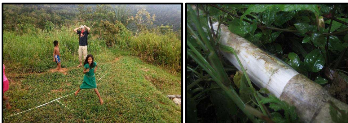
Figure 3: (Left) A pipe running above ground on a common path between homes in the community. (Right) A leaking pipe due to improper sealant.
