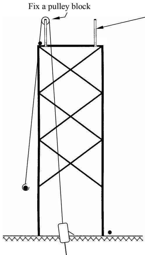
Temporary device for lifting the main cables (supplied with Top Element)
