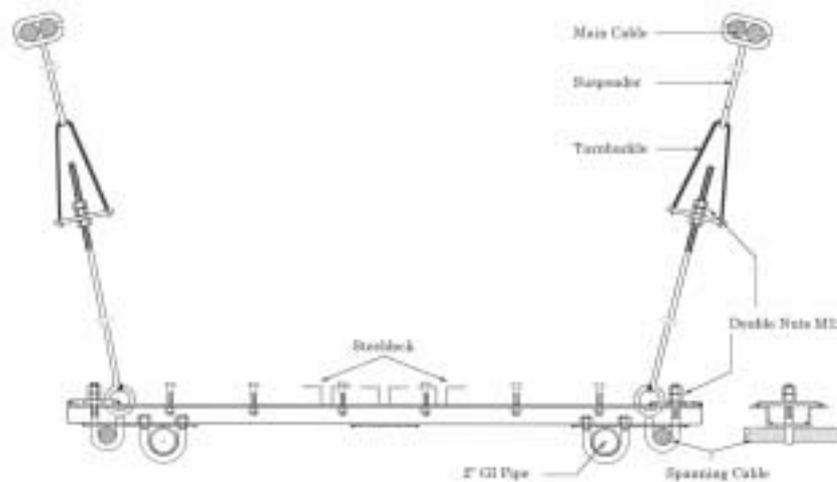
The G.I. pipes have to be fitted before the outer rows of the steel decks are mounted in the following way:
