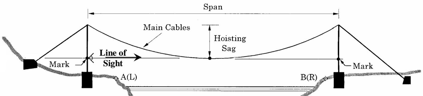
Also check the sags from time to time when the fitting works are going on. Different elongations may take place due to dissimilar hidden cable relaxations when the tension increases. Adjust possible sag differences with the help of the turnbuckles at the main cable anchor so that the Main Cables are always parallel and compare the dead load sag with the pre-calculated values.
