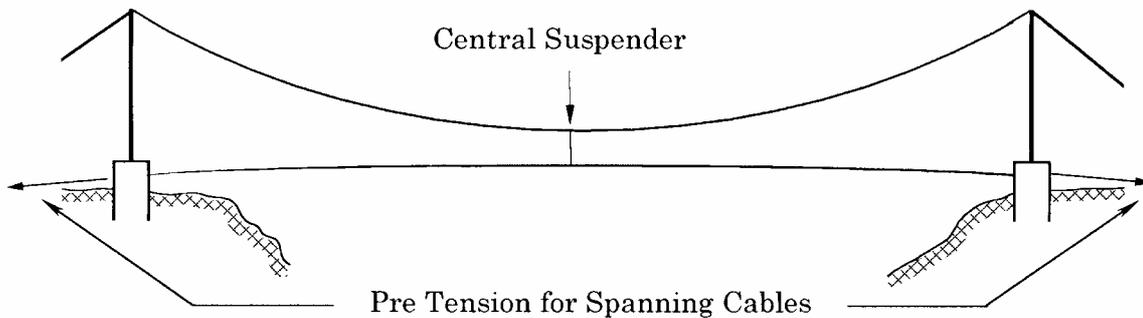
Tighten the spanning cable to some extent; now the cables are ready to be fixed to the suspenders.
