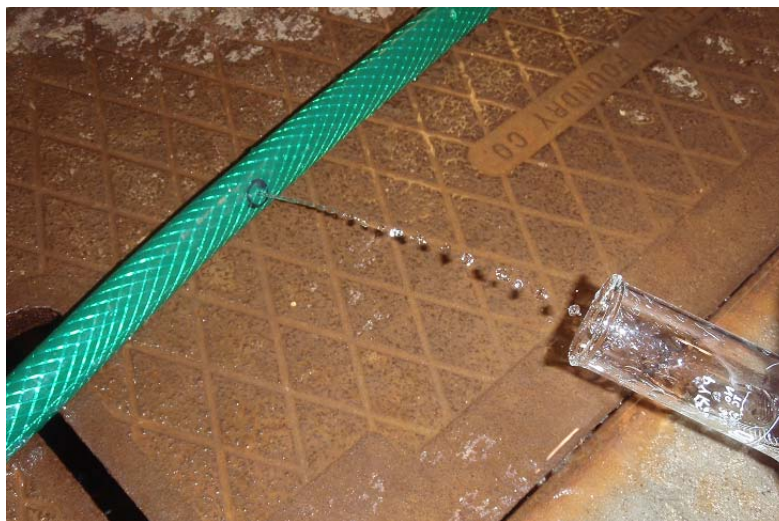
Figure 8: Flow Testing of Irrigation System
