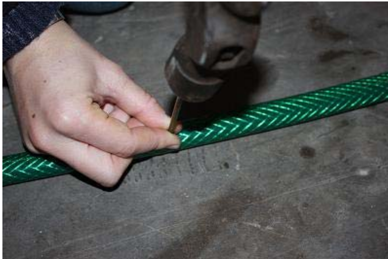
Figure 7: Creating Emitter Holes in Irrigation Lines
