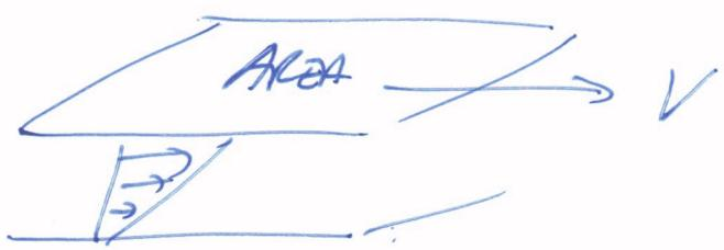
$$\text{Shear stress} = \frac{\text{Force to pull plate at } V}{\text{AREA}}$$
