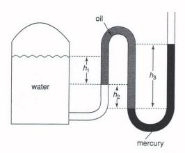
We use the static-pressure relationships to relate pressure in a tank to the various heights of fluids as shown (Problem 17).
