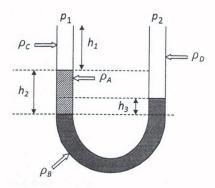
A schematic of a manometer that contains two different measurement fluids (Problem 16).
