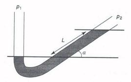
Schematic of a tilted manometer (Problem 15).
