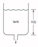
Schematic of a tank draining. This problem is solved with the mechanical energy balance and quasi-steady-state methods (Problem 44).
