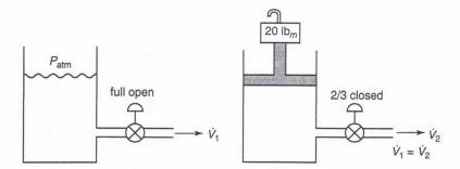
Water drains from two tanks at the same rate. However, the tank is open to the atmosphere in one case; in the other case, an external pressure is imposed as shown (Problem 43).
