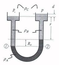
If more top fluid is present on the left than on the right, the initial reading of a double-well manometer is  $R_0$  (Problem 18).
