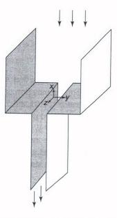
Planar contraction flow occurs when a larger reservoir drains through a slot (Problem 32).
