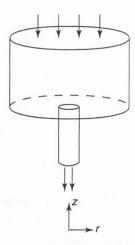
Axisymmetric-contraction flow occurs when a larger round reservoir drains through a pipe (Problem 33).
