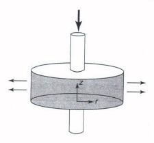
Squeeze flow between two parallel plates is a common flow test geometry (Problem 31).
