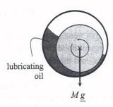
Schematic of a lubrication flow. The central axis may be the axle of an automobile, for example, and the outer ring represents part of the housing.
