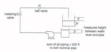
To choose a pump for the system shown (Problem 31), a system-head curve is constructed.
