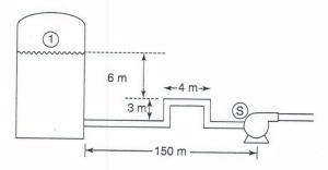
Avoiding cavitation in an installed pump (Problem 35).
