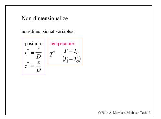
$$h(\pi \mathbf{D}L)(T_1 - T_0) = \int_{0}^{2\pi} \int_{0}^{L/D} -k \frac{\partial T^*}{\partial r^*} \Big|_{r^* = 1/2} \frac{(T_1 - T_0)}{D} \frac{\mathbf{D}}{2} dz^* d\theta$$
