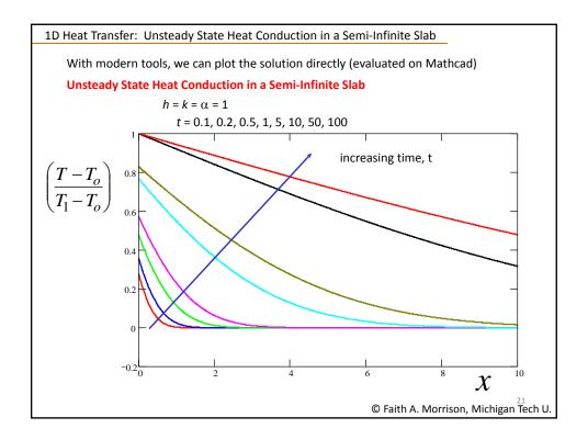
1D Heat Transfer: Unsteady State Heat Conduction in a Semi-Infinite Slab
