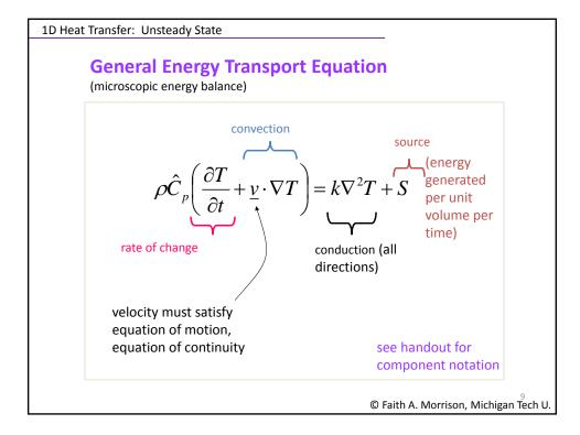
**Equation of energy** for Newtonian fluids of constant density, ρ, and thermal conductivity, k, with source term (source could be viscous dissipation, electrical energy, chemical energy, etc., with units of energy/(volume time)).
