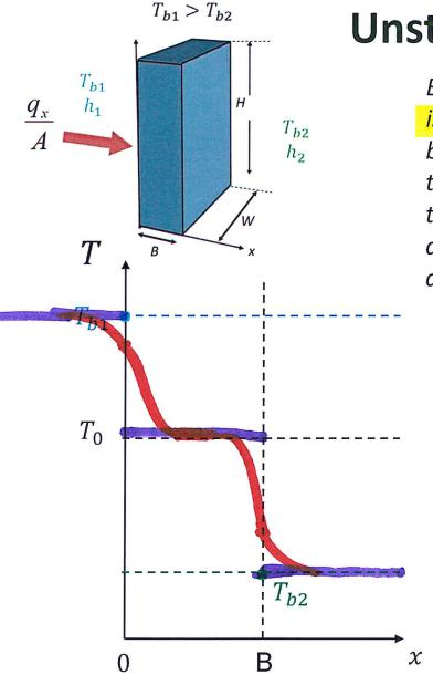
Example: A wide, tall slab initially uniformly at  $T_0$  is suddenly subjected to flowing fluid on its two broad faces. The left fluid is at  $T_{b1}$  and its heat transfer to the wall is characterized by heat transfer coefficient  $h_1$ , while the right side is at  $T_{b2}$  and characterized by  $h_2$ . What is the temperature distribution across the slab as a function of time?
